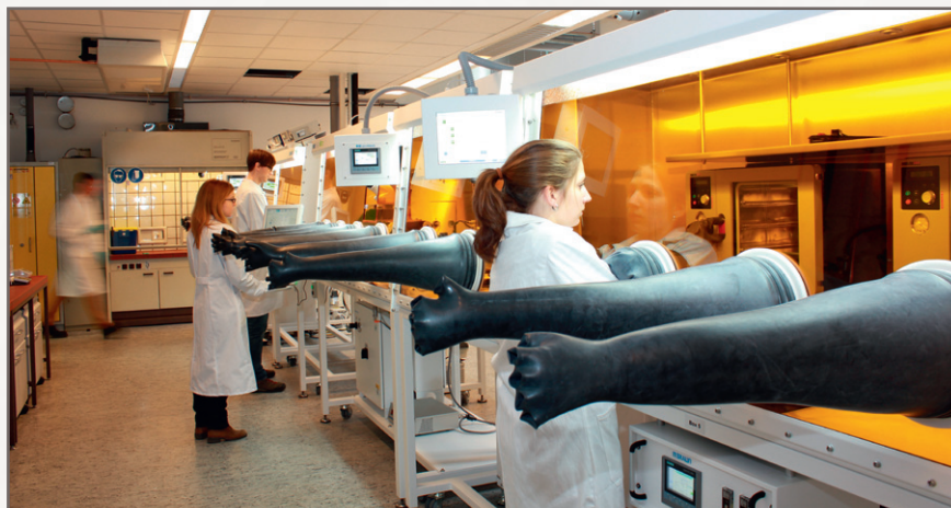
Argon box prototyping line for substrate integrated lithium micro batteries.
